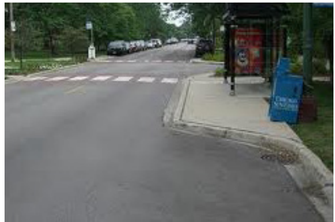
Curb extension or bulb-out
